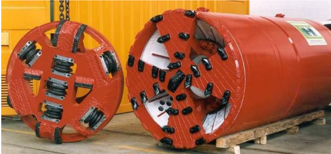
Figure 6. Two MTBM Cutter Head Options. Disk Type Cutters on Left for Rock, Drag Bits for Clay/Silt on Right
